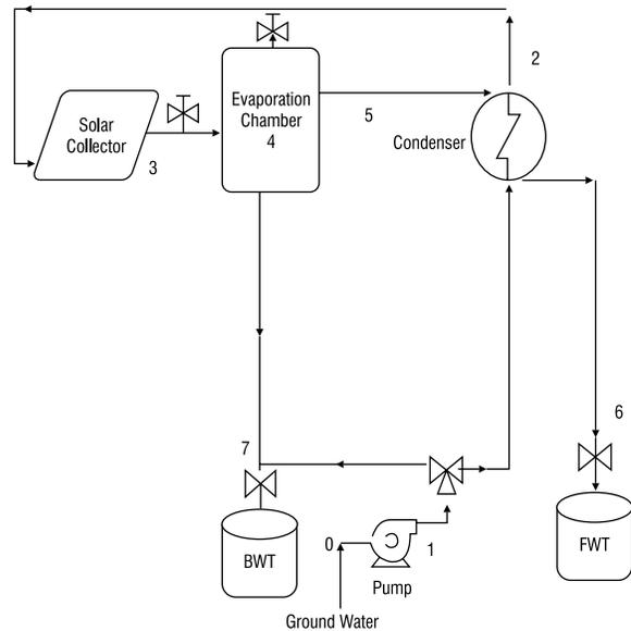
**Fig. 4: Process pattern of desalination system**
