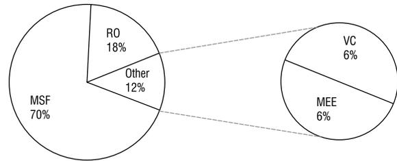
**Fig. 3: Market share of different seawater desalination technologies<sup>1</sup>**
